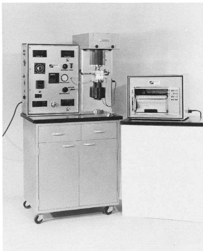
FIG. 2 Falex Variable—Speed Four-Ball Wear Test Machine
